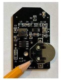
Remove the board from the case and push the old battery out from the side. Avoid contacting electrical components. (This is a good time to inspect the battery contacts and clean if necessary). Install the new battery <u>+ side UP</u>.
